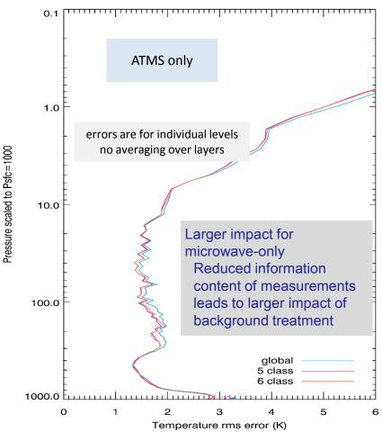
500 profiles from simulated measurements
