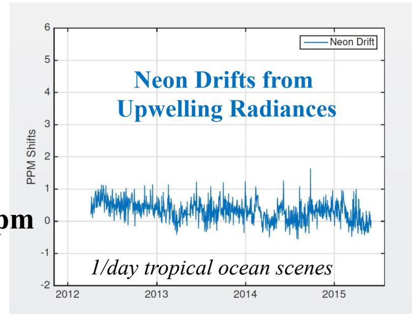
**Variation of FTS effective metrology laser wavelength calibrated with stable onboard Neon source reduces final error to < 1 ppm!**
