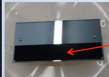
Lithographically defined spectrometer slit with black Si anti-reflection surface fabricated for OCO2
