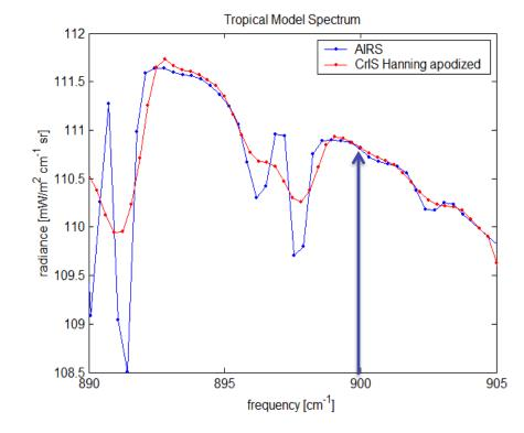
We bypass the SRF normalization and resampling problem by analyzing one channel in the broad atmospheric window region near 900 cm<sup>-1</sup>. The difference here is less than 50 mK.
