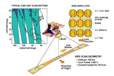
Figure 3: AIRS scanning and coverage geometry.
