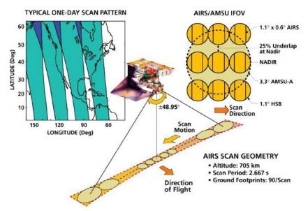
Figure 3: AIRS scanning and coverage geometry.
